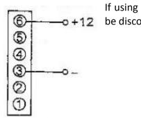
If using external power,voltage DC1V,current ≥ 1A.Control terminal ① must be disconnected with power N side,other connection remains.
